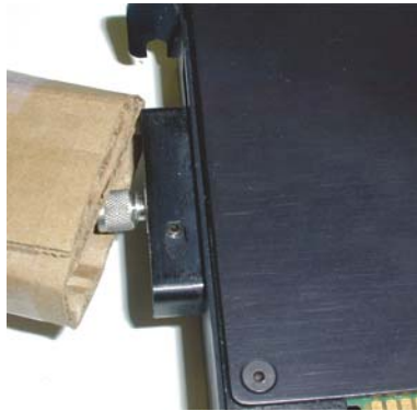
Figure 4: Insert the folded cardboard (B) over the fiber optic cable connector to protect it during shipment.
