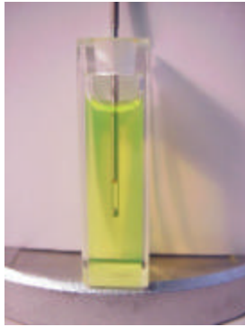
Fig.10: Miniaturized dipping-probe in a 10mmx10mm cuvette
